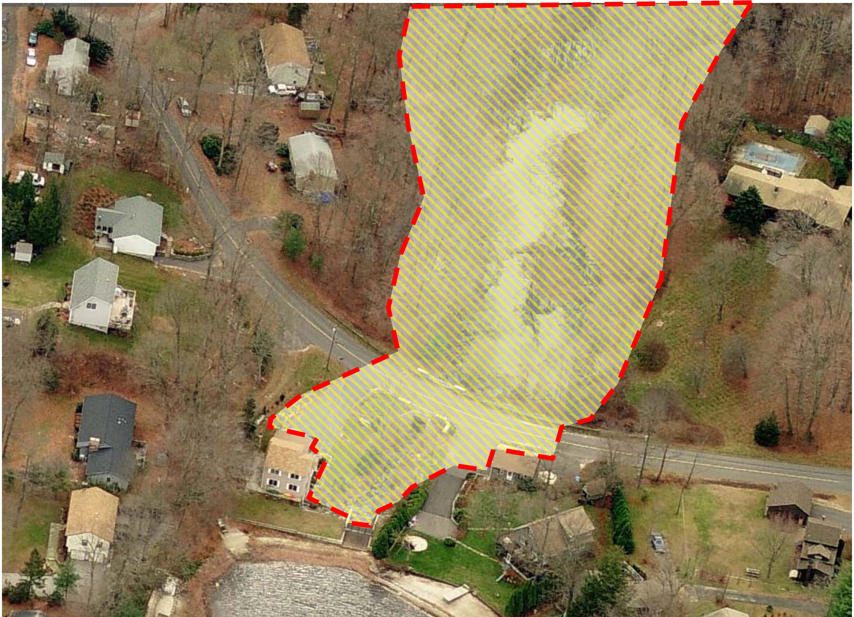
Figure 2 – Breach inundation area looking in a southerly (downstream) direction from the pond and dam.
